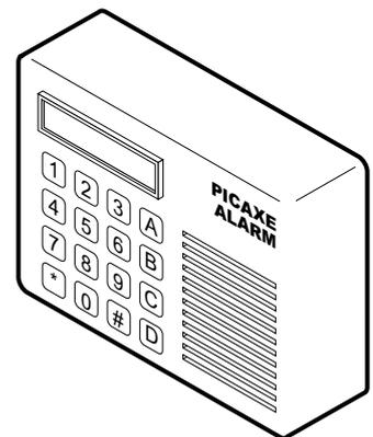
In the case of a fire alarm system the inputs may be smoke sensors and the keypad on the front of the control panel. The output devices are the display on the control panel as well as the external siren and strobe light. The microcontroller is the 'brain' of the system.
