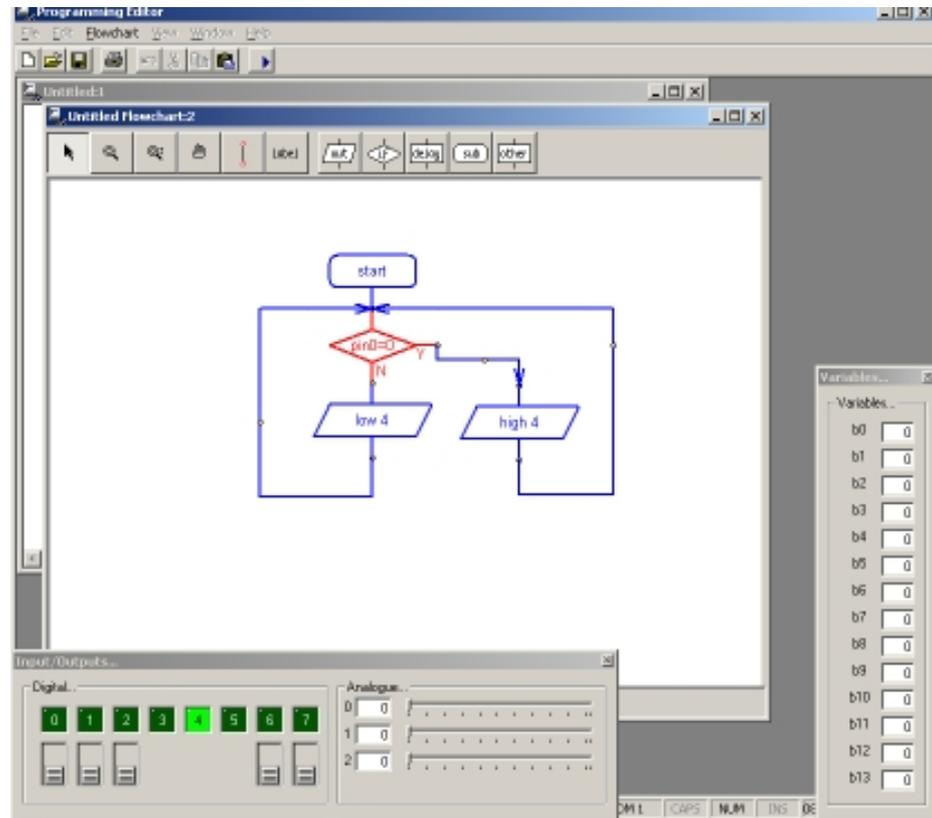
To simulate the flowchart, click 'Simulate' from the Flowchart menu. The program will then start to run on-screen.
