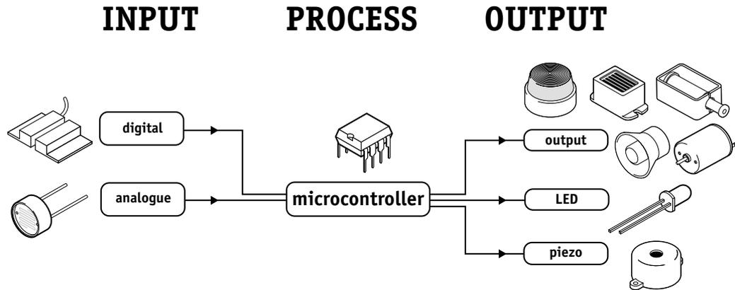
The project can also react to digital and/or analogue sensors (e.g. an LDR light sensor).
