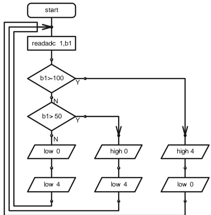
The 'readadc' command is used to read the analogue value (a number between 0 and 255) into variable b1. Once the number is in variable b1 it can be tested to see if it is greater than 100 or greater than 50. If it is greater than 100 output 4 is switched on, if it is between 50 and 100 output 0 is switched on, and if it is less than 50 both outputs are switched off.
