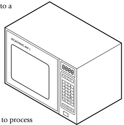
As an example, a microwave oven may use a single microcontroller to process information from the keypad, display user information on the seven segment display, and control the output devices (turntable motor, light, bell and magnetron).
