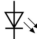
The positive (anode) leg of an LED is longer than the negative (cathode) leg (shown by the bar on the symbol). The negative leg also has a flat edge on the plastic casing of the LED.
