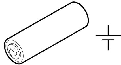
Microcontrollers generally require 3 to 6V to work, and so it is better to use a battery pack made up of three or four AA size cells. Never use a 9V PP3 battery as the 9V supply will damage the microcontroller.
