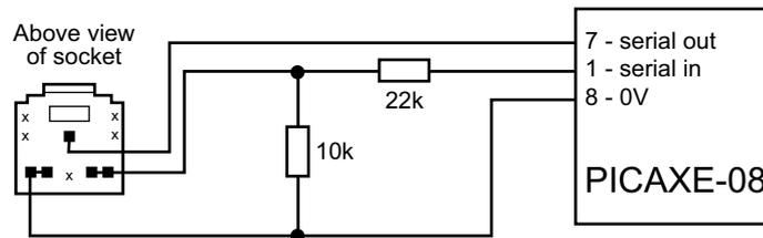
The socket and interfacing circuit is included on every PCB designed to be used with the PICAXE-08 microcontroller. This enables the PICAXE microcontroller to be re-programmed without removing the chip from the PCB - simply connect the cable whenever you want to download a new program!
