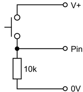
When the switch is activated, the input pin is connected to the positive battery supply (V+). This provides an on (logic level 1) signal to the microcontroller.
