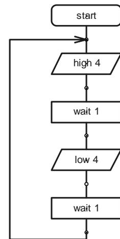
This program would switch the buzzer (connected to output pin 4) on and off every second. If the buzzer does not sound check that:
