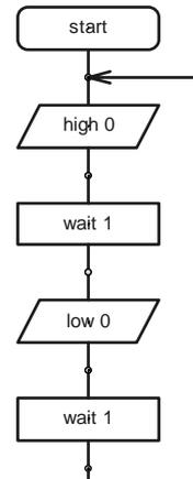
The LED should flicker as the program downloads. After the download is complete the LED should flash on and off every second. If the LED does not flash check that it is around the correct way and that the 330R resistors are in the correct positions on the PCB.
